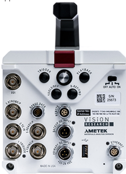
The Phantom T4040 rear panel features trigger input ports as well as a physical button to trigger.
