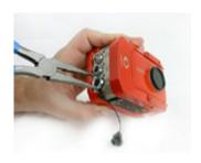
Position the needle nose pliers into the teeth of the locking collar and firmly tighten the collar.
